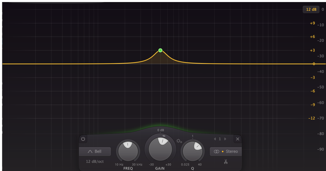
FIGURE 8 - BOOST WITH IDENTICAL PARAMETERS APART FROM Q RAISED TO 3 FROM 0.5
